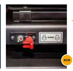
**Emergency stop switch** The engine can be shut down immediately using an emergency stop switch located at the base
