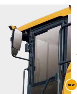
Foldable side mirror The side mirror is easy to adjust for optimal visibility and can be folded away to prevent damage during transportation.
