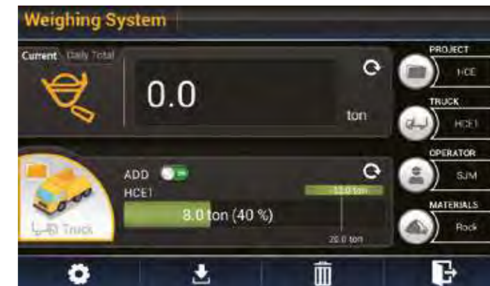
The highly accurate automatic/manual cumulative weighing system helps you to manage production more efficiently in any environment. For maximum precision, weighing error icons and a two-colour weight value indicator are displayed on the monitor.
