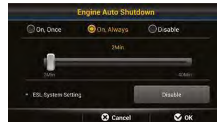
The engine shuts down automatically when the machine is at rest to cut fuel consumption and prevent unnecessary emissions. Different operating modes and idling times can be selected according to the work environment, further enhancing efficiency.
