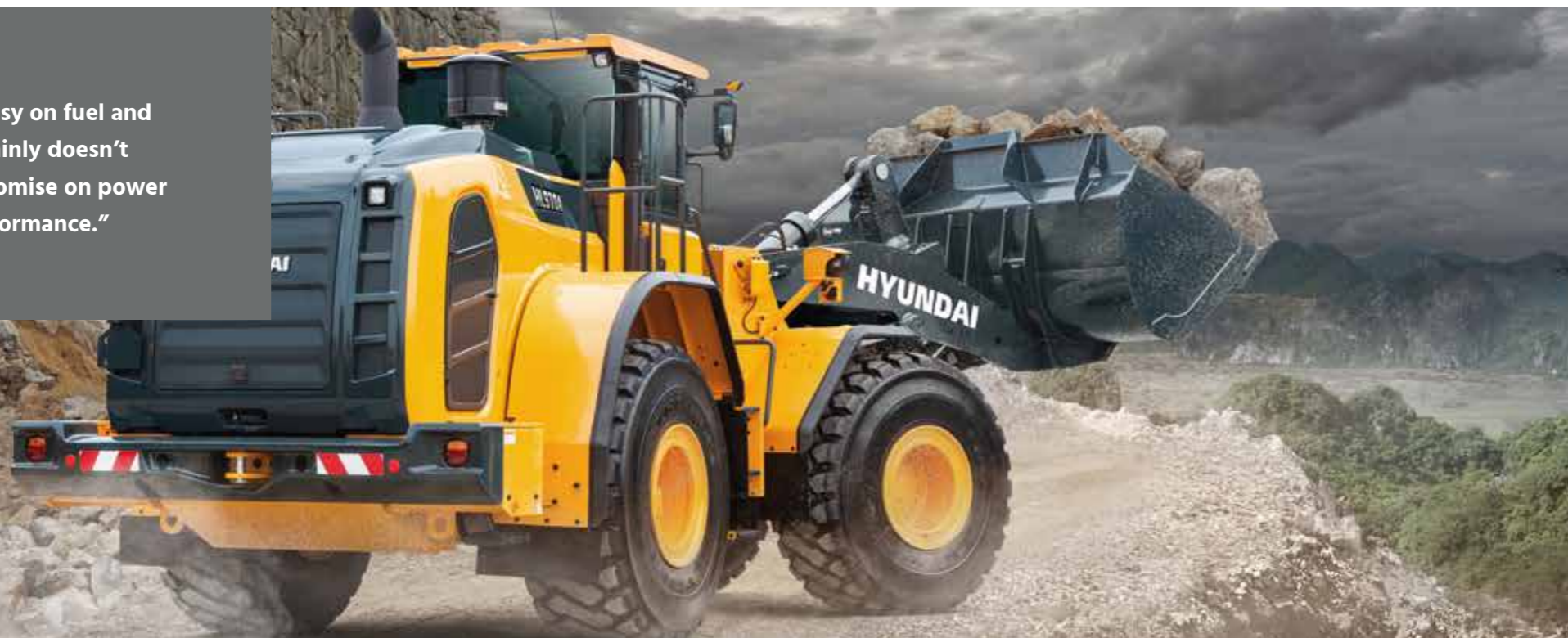
The new Smart Power mode adjusts engine RPM in heavy load work like digging to save fuel without compromising on performance. The technology also achieves an optimal balance between traction and breakout forces.
