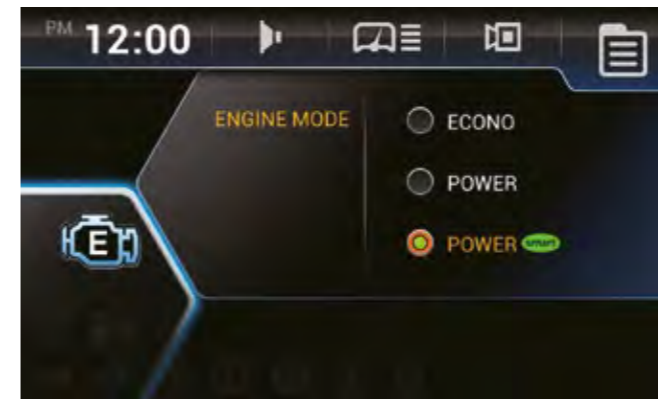
The new Smart Power mode adjusts engine RPM in heavy load work like digging to save fuel without compromising on performance. The technology also achieves an optimal balance between traction and breakout forces.
