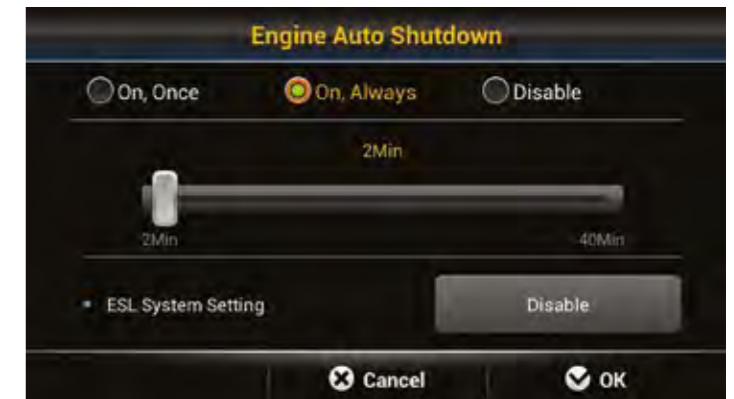
The engine shuts down automatically when the machine is at rest to cut fuel consumption and prevent unnecessary emissions. Different operating modes and idling times can be selected according to the work environment, further enhancing efficiency.
