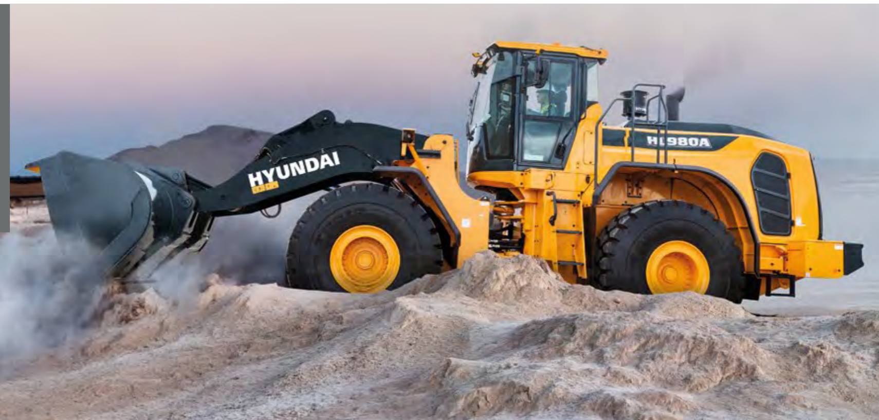
The new Smart Power mode adjusts engine RPM in heavy load work like digging to save fuel without compromising on performance. The technology also achieves an optimal balance between traction and breakout forces.
