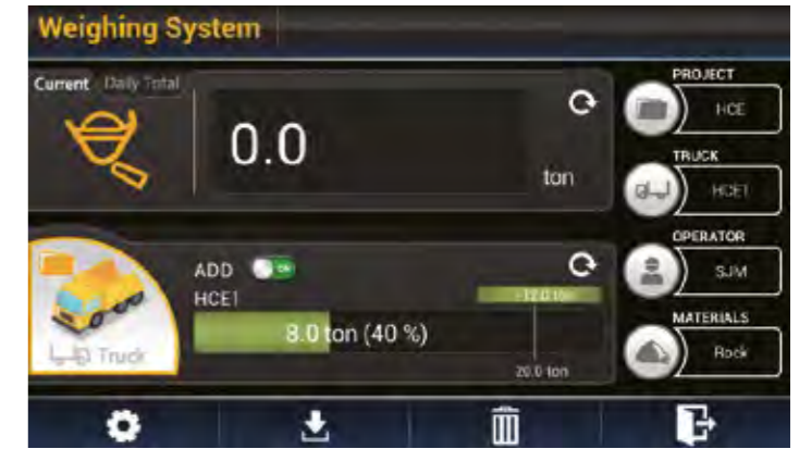
The highly accurate automatic/manual cumulative weighing system helps you to manage production more efficiently in any environment. For maximum precision, weighing error icons and a two-colour weight value indicator are displayed on the monitor.
