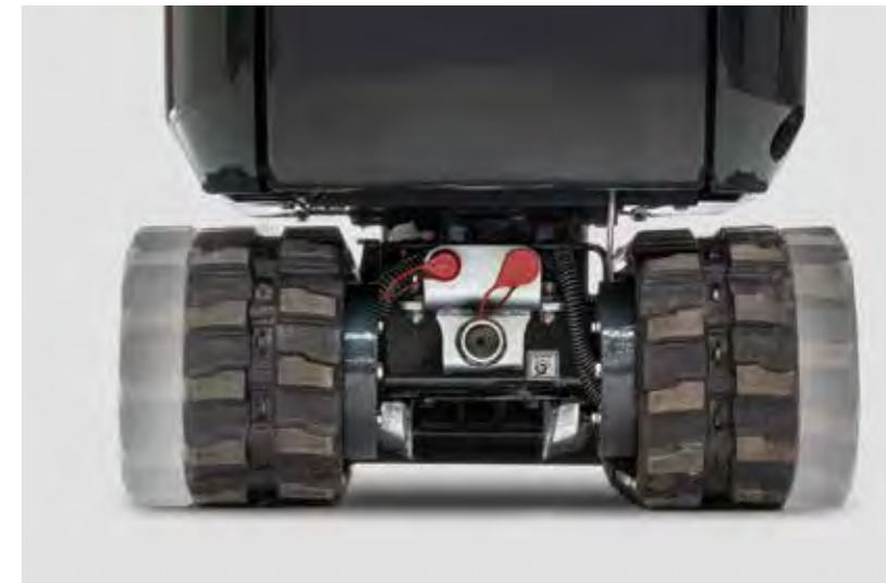
The variable undercarriage guarantees trouble-free passage through doors, corridors and alleyways
