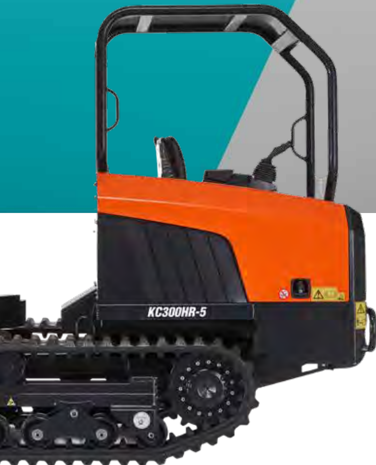
KC300HR-5 (180° rotary dumping function)
