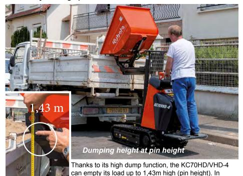
addition, the dumping reach of 447mm allows easy
