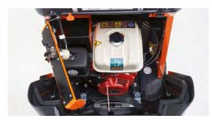
The console of petrol version can be opened for easily refueling of tank. In the diesel version, the operation is equally easy to accomplish.
