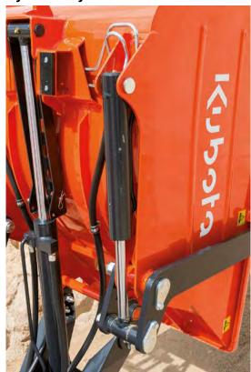
The loading shovel is activated by two hydraulic cylinders located under the skip. Due to their position, they are well protected and they ensure a good lifting capacity.
