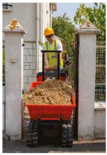
Like the other models of the product family, the Kubota KC70HD/VHD-4 has been designed to work in confined area. The variable undercarriage version allows it to be driven through narrow spaces when minimum width is set (758mm overall width) and insure excellent stability when the undercarriage is extended to the maximum position (1058mm).
