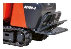
The KC70-4 features a foldable foot plate. When the plate is down, the operator can safely stand on it to operate the machine. When the plate is folded up, the overall length is reduced by 214 mm in order to gain space for transport or storage. The standing operation position makes it easier when getting on and off the machine.
