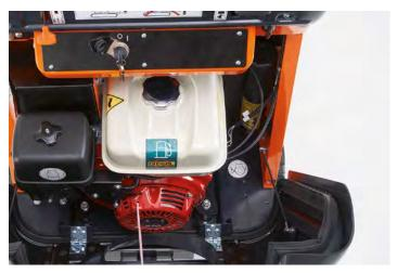
A large opening bonnet gives good access to the main areas for daily maintenance: fuel tank, air filter, engine oil level, battery, and battery isolator switch (when present) are easily reachable.
