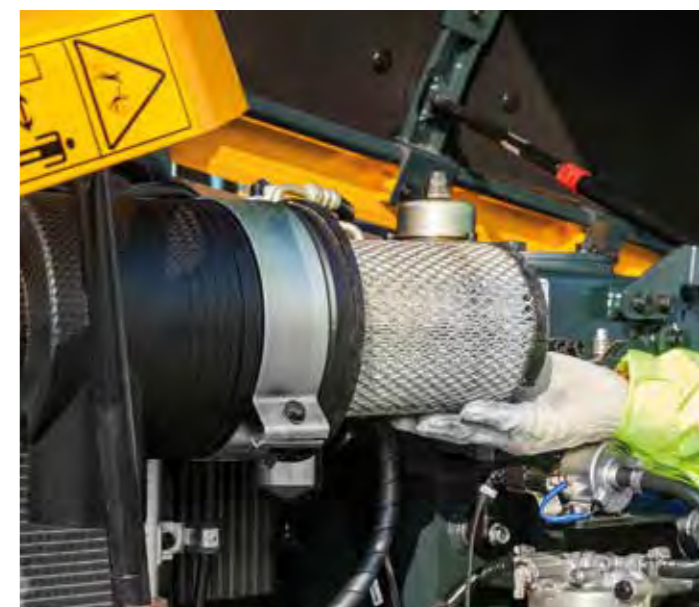
Air filter The R18-9AK is fitted with a durable plastic air filter designed for easy maintenance.
