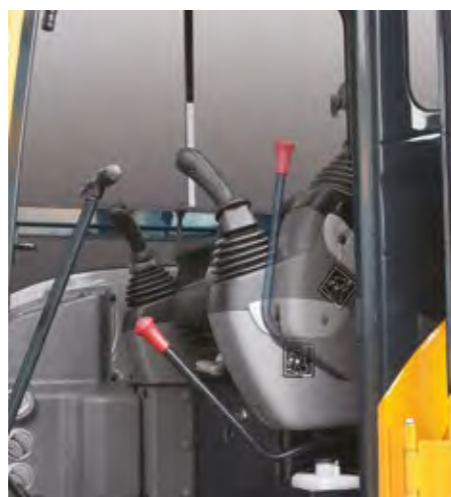
Safety lever A safety lever is installed to prevent unintentional activation of the hydraulic attachments. When the safety lever is positioned upright, hydraulic functions are disabled.
