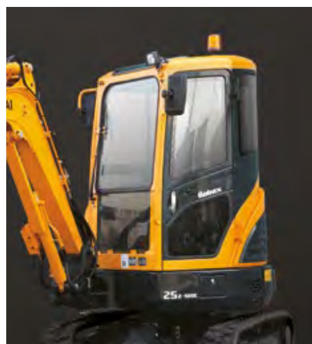
Cabin The operator is protected by a robust cabin structure, built using strong, slim tubing to optimise both sturdiness and visibility. The canopy and cabin frame comply with international TOPS, ROPS and FOG standards.
