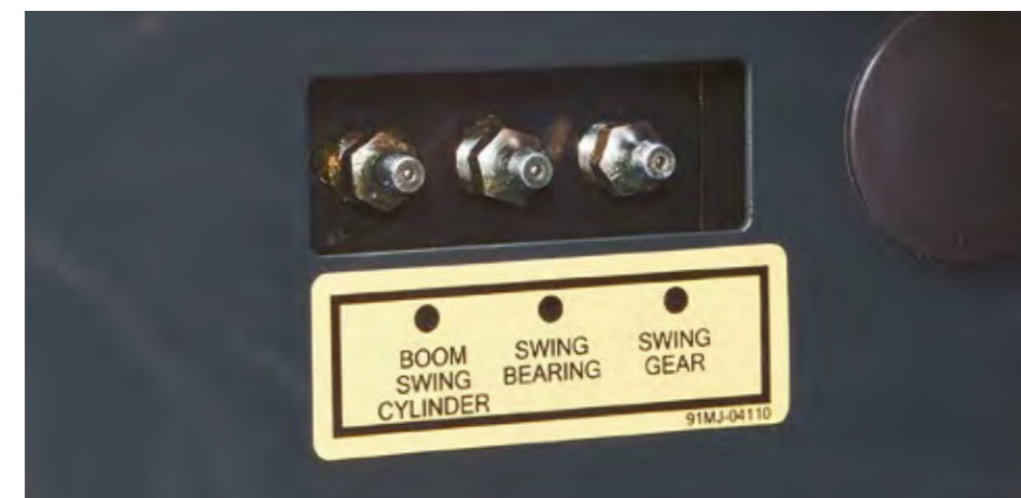
Centralised grease fittings The lubrication bank centralises grease fittings for quick, easy servicing.
