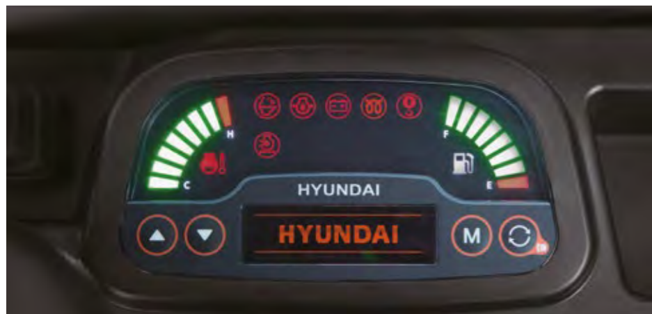
Indicators and gauges An array of gauges and warning indicators are displayed on the monitor. The monitoring system allows you to check machine status at a glance and includes an hour meter, oil pressure lamp, battery change lamp, engine coolant temperature gauge and fuel gauge.
