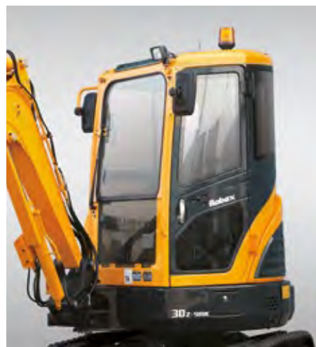
Frame The operator is protected by a robust cabin structure, built using strong, slim tubing to optimise both sturdiness and visibility. The canopy and cabin frame comply with international TOPS, ROPS and FOPS standards.
