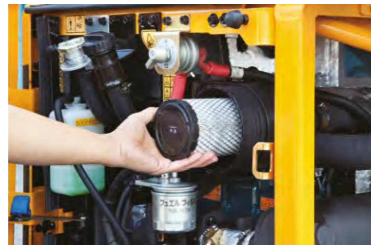
Air cleaner The durable air cleaner is designed for convenient maintenance.
