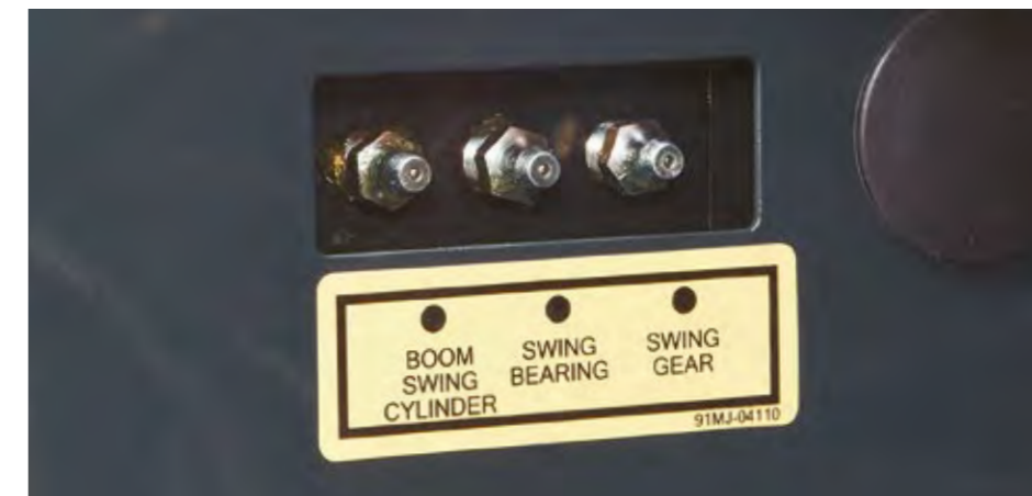
Centralised grease fittings The lubrication bank centralises grease fittings for quick, easy servicing.
