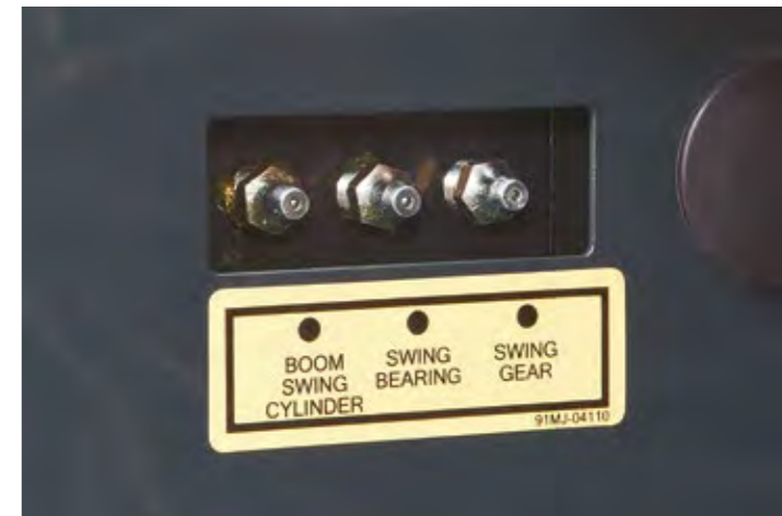
Centralised grease points Grease fittings are centralised in one lubrication bank for quick, easy servicing.
