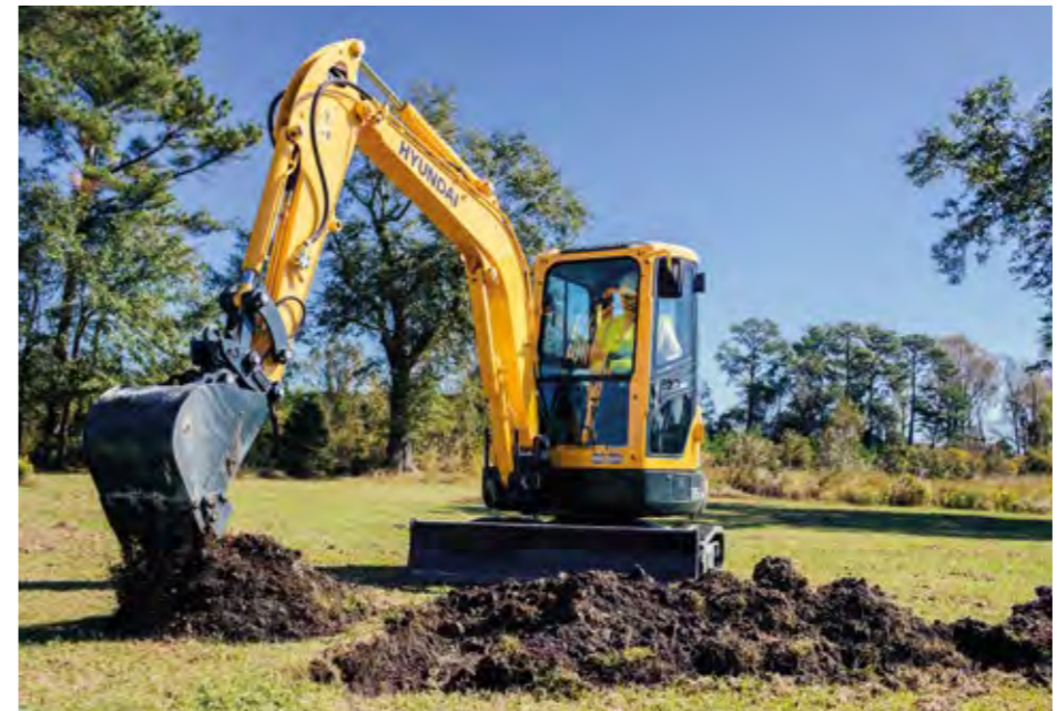
Auto shift down system When working under heavy load or when the machine is climbing a slope, the travel motor speed automatically shifts down into first gear. This increases the tractive effort and the travel motor will automatically switch back into fast gear once the load is reduced.
